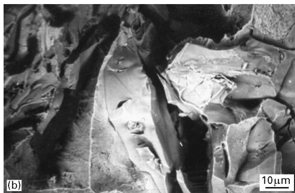
Figure 5 The microstructure of fracture observed by SEM (a) the panorama of the fracture surface (b) the microstructure of the solder peeled off the ceramic.
